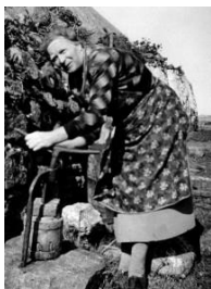
1997.179.10 Isabella MacLean was photographed using a cheese press in Kilmoluaig by George Holleyman, an archaeologist posted to RAF Tiree during World War II. The press was made in the local smiddy. The screw, which turns through an iron hoop set into a large stone, tightens on to the wooden cheese vat, removing excess whey. The cheese press is part of An Iodhlann`s collection.
