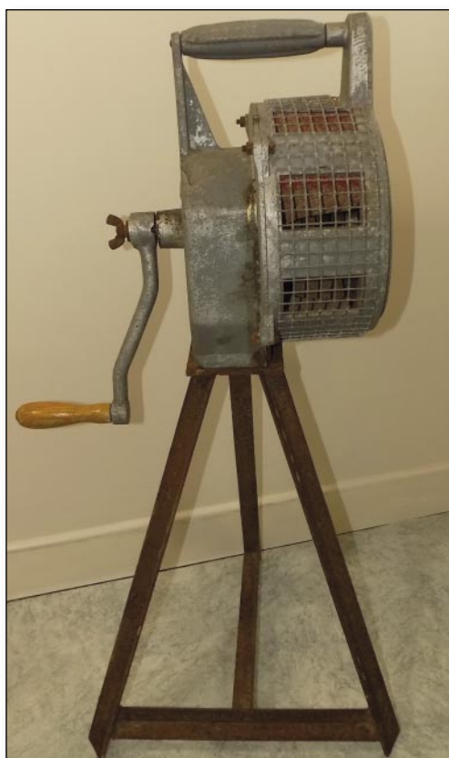
Carter hand operated siren (left), part of the equipment on Tiree during the Cold War. Household leaflet (right) illustrating survival techniques following a nuclear blast.
