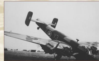
This Halifax overtook the runway at Tiree and tipped into a ditch
